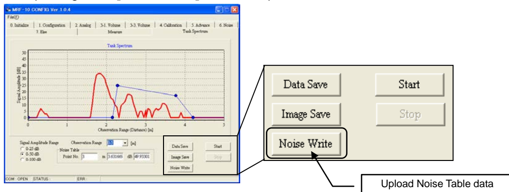
Fig. 4.8-4 Uploading of Noise Table data
